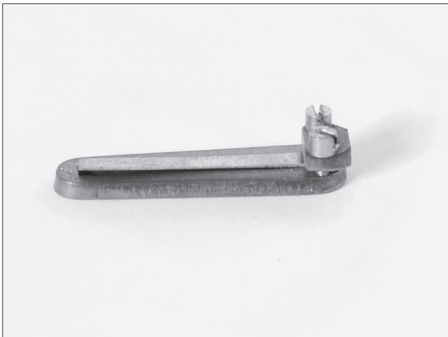
(a) A reed mounted in a frame (its aperture visible as the dark grey area below it)
